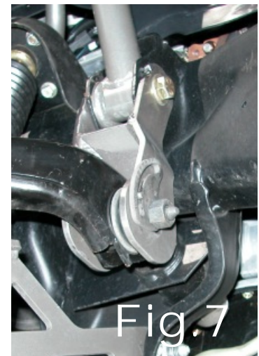
Upper A-Arm drop bracket with Dual Shock Hoop Installed .
