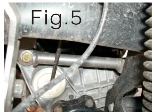
Driver Side Differential Support Rod
