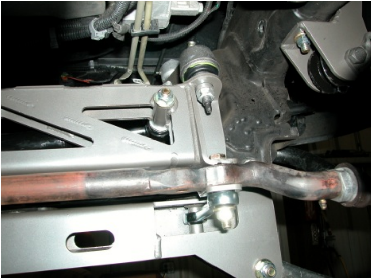
Front and rear subframes, steering center link and factory bump stops installed.
