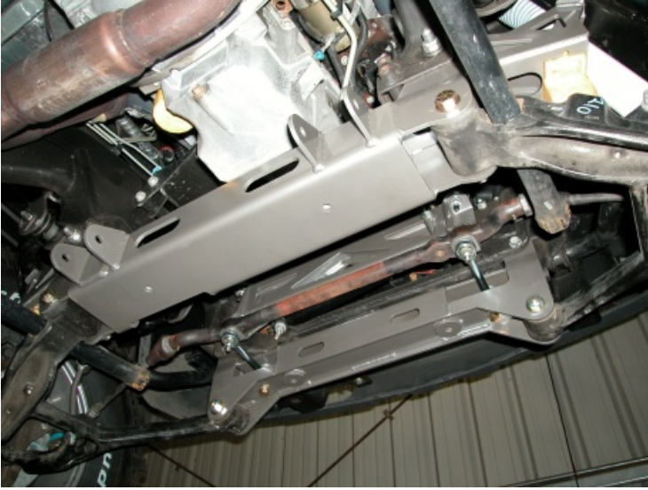
Front and rear subframes, steering center link and factory bump stops installed.
