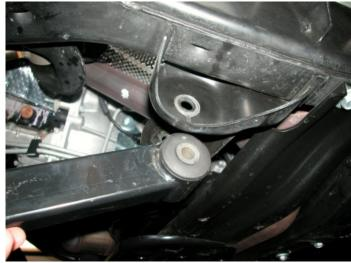
Remove factory control arms from frame and axle.
