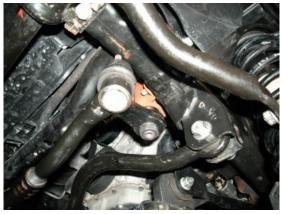
Disconnect front track bar from axle. It is not necessary to disconnect it from Fig.2 the frame as shown.
