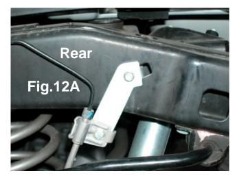
8. Using the factory bolt located on the frame, install new left and right rear brake line extension brackets as shown in Fig.12A & 12B
