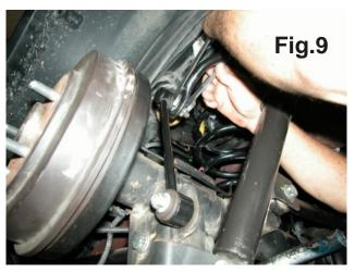
2007 Rubicon models come factory equipped with electric sway bar disconnect. Remove the factory rear sway bar links and install them on the front sway bar. Caution: DO NOT USE Full-Traction Sway Bar Disconnect Links on the Front Rubicon sway bar.
