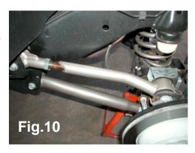
torque. This method eliminates torque twist to the rubber bushings. Torque bolts per factory specifications.
