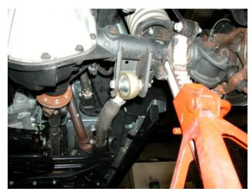
Fig 8 shows the radius of the new arm and proper mounting. (Left/Driver side shown)
