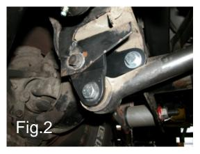
**5.** Leaving the spring attached to the frame of the vehicle, remove the center bolt on the spring holding the leaf pak together.
