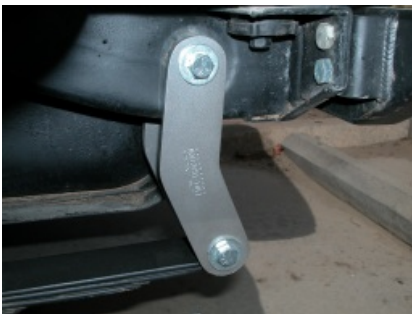
Rear (YJ shown) CJ Shackles mount to the OEM spring hanger on the bottom of the frame.
