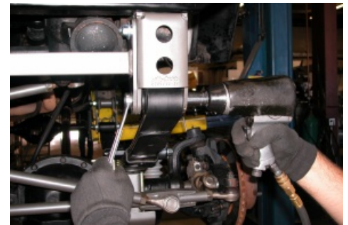
Installing Front Shackle Tower with cross brace.
