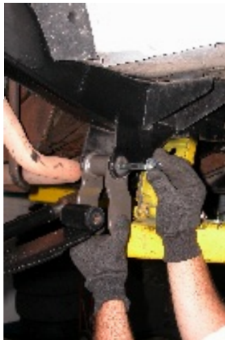
Installing Bell Shackle on the rear of the front spring.
