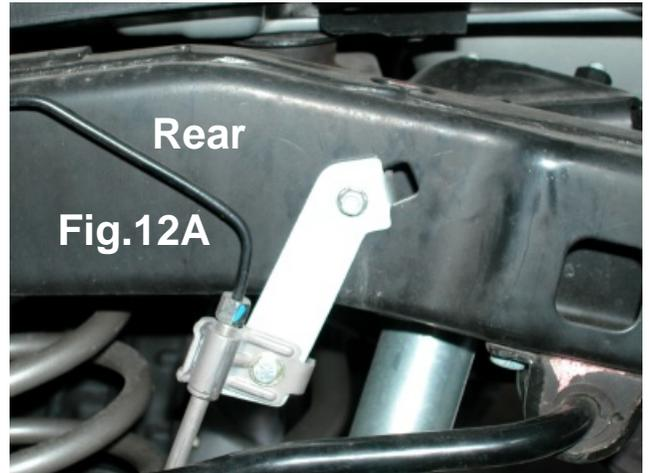
8. Using the factory bolt located on the frame, install new left and right rear brake line extension brackets as shown in **Fig.12A & 12B**
