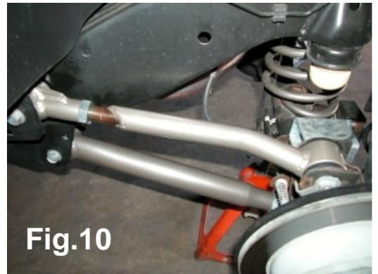
5. Before installation, assemble new Full-Traction rear track bar. Install new Vecton material bushings and SLE105 sleeve into eyelet. Bushings must be press fitted with a bench vise or H-press. Bushings are brittle and should not be hit with a steel hammer. Install new Heim joint and jam nut into threaded end of track bar. Install new
