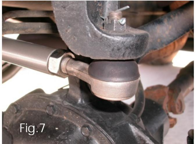
2. Proper installation of **ES2223R** tie rod end is very important. Install the 11/16 Lock Nut onto the treads of the new tie rod end. Install the tie rod end all the way into the track bar threads. There must not be more than 3-4 threads showing outside the lock nut as shown in **Fig. 7 Install nut and cotter pin as shown.**
