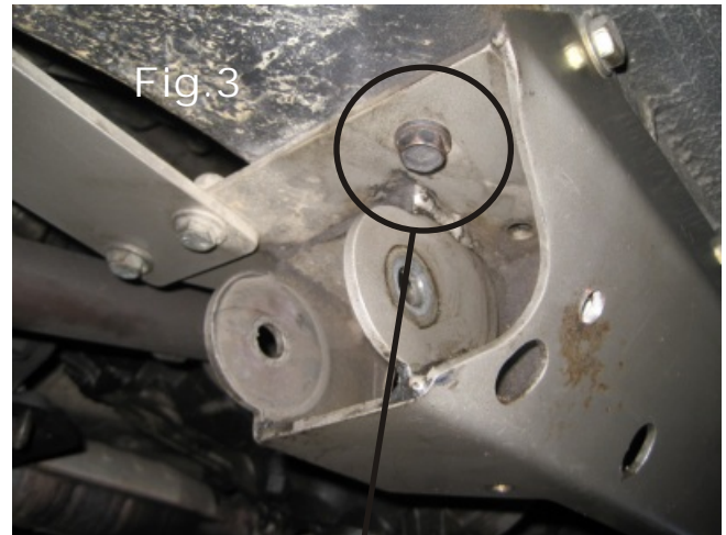
Factory frame reference hole
