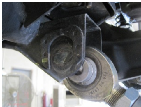
Lower Front Control Arm being attached to front axle.
