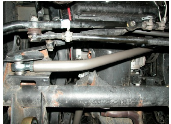
Front Track Bar Mis-Alignment Spacers Installed
