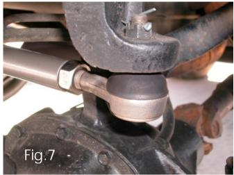
3. It is mandatory to install and adjust the front track bar while vehicle is on the ground.
