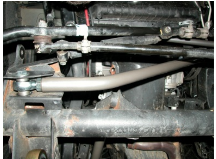
Front Track Bar Mis-Alignment Spacers Installed
