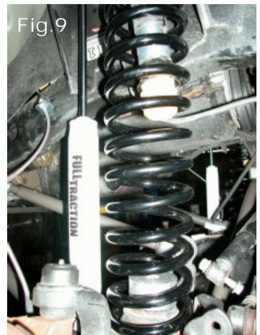
Front Coil Springs with bump stop extensions correctly installed.
