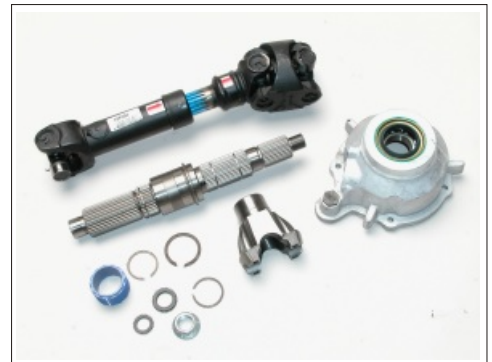
Typical Rear CV Drive Shaft & Slip Yoke Eliminator
